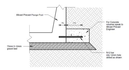
Anti-floatation control is only required for in-ground pools. Speak to Allcast Precast for details.
